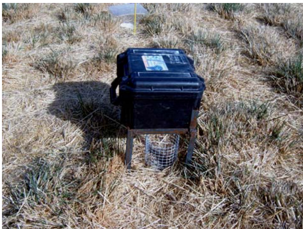
Time lapse camera placed over a seed station in a tall fescue field in 2006 (pitfall traps are located in the background), and one image from a time lapse movie of a ground beetle visiting a seed station with Powell amaranth seeds.
