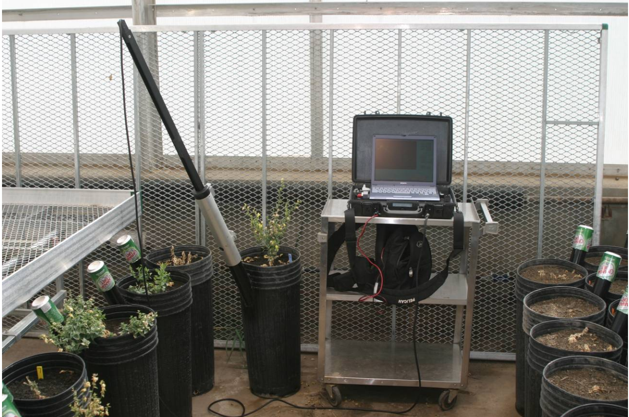
Figure 2. The minirhizotron system. The camera is attached to an indexed handle and is inserted into a clear acrylic tube through the side of the container. Root images are captured and stored on a portable laptop computer for analysis with imaging software.
